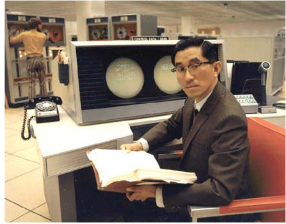
Akira Kasahara (ca. 1967) at the console of the NCAR cdc 6600 computer. The 6600 had a clock speed of 10 MHz and a memory of 64 KBytes and was the fastest and biggest computer devoted to meteorological studies at the time.
